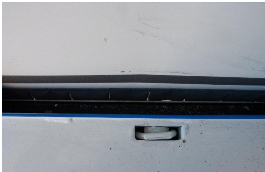
Figure 2.6: Tarpaulin with pleated skirt sealing (opened)
