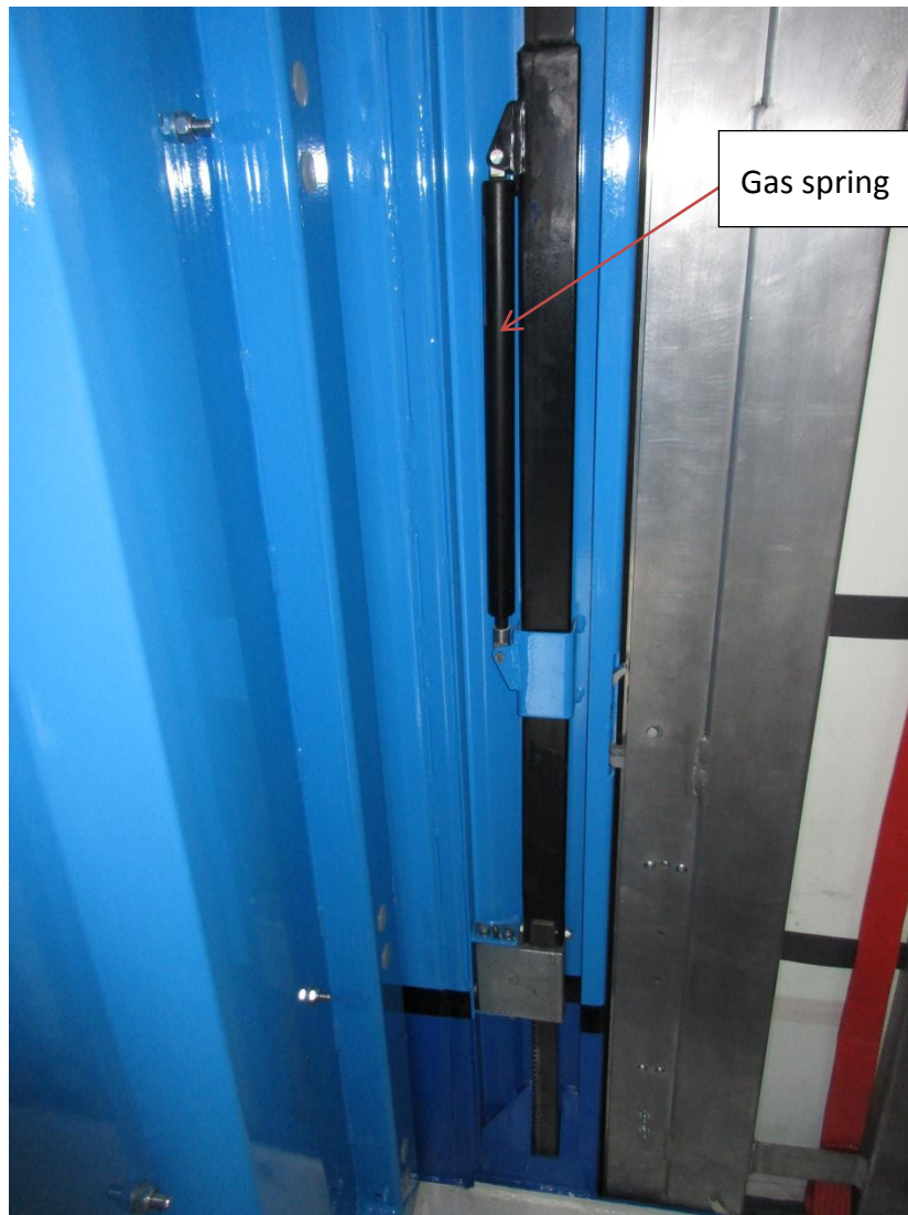
Figure 2.5: Roof lifting system with additional gas spring
