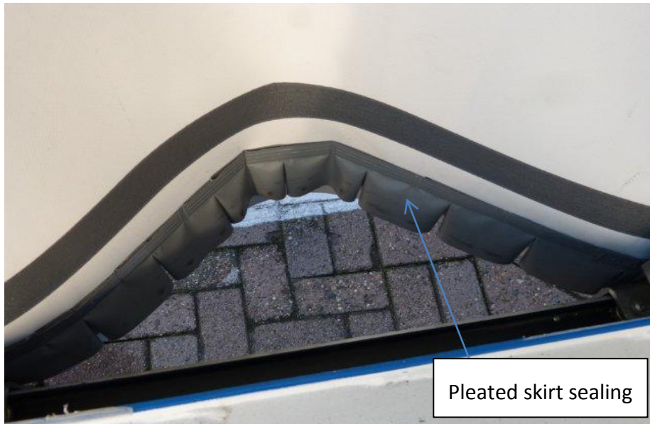
Figure 2.6: Tarpaulin with pleated skirt sealing (opened)
